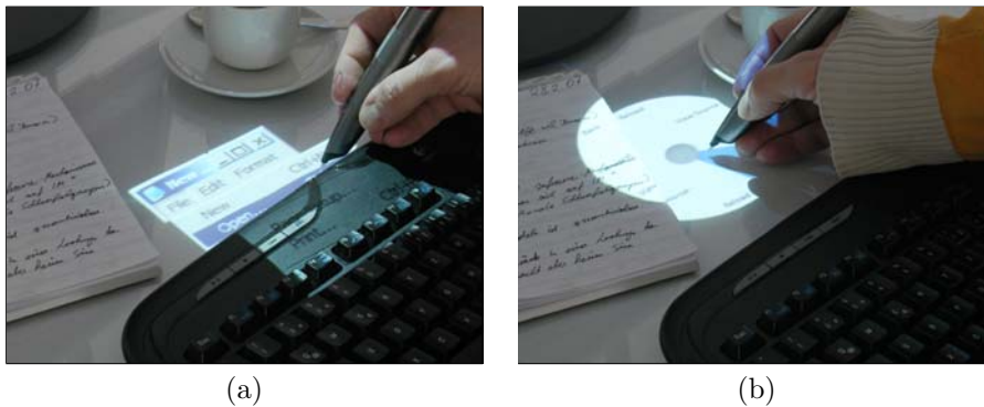
Figure 5.4: Drop-down menus (a) and pie menus (b) become hard to see or even unusable when overlapping with physical objects on a tabletop display.
