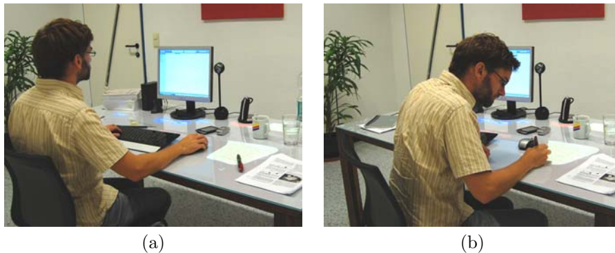
Figure 4.1: Pentable interfaces. Standard PC interfaces like keyboard, mouse and LCD screen are used for most tasks, while the tabletop display presents ambient information (a). For tasks requiring pen-based interaction, the user focus shifts to the tabletop interfaces (b).
