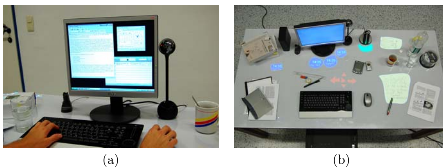
Figure 5.1: The PenTable LCD display shows a standard WIMP GUI (a), while the characteristics of the tabletop display require a special GUI (b).
