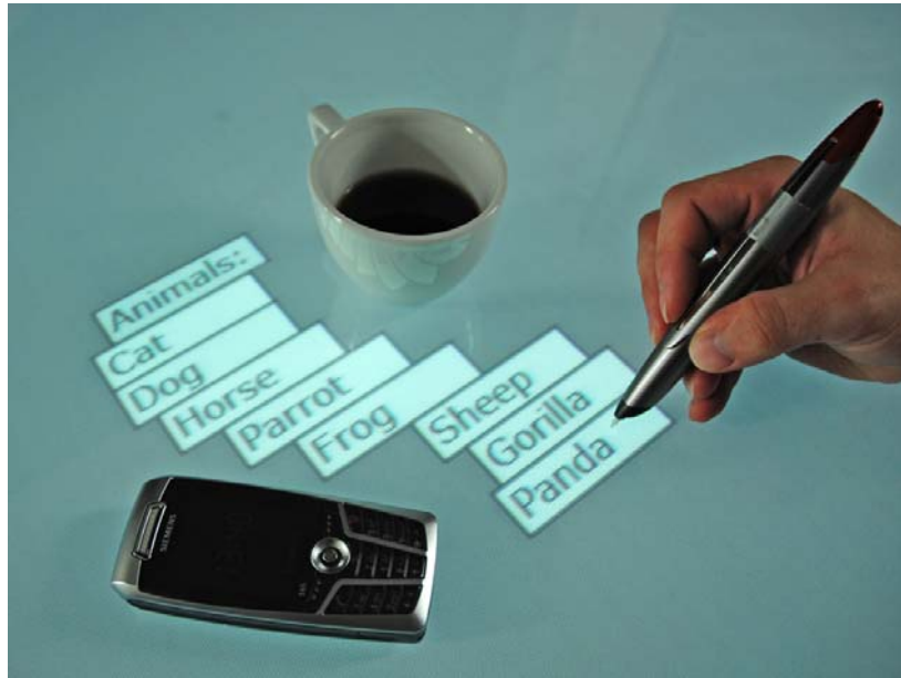
Figure 5.5: The menu items of a pMenu are placed along a user-drawn path to avoid occluding objects on the tabletop.
