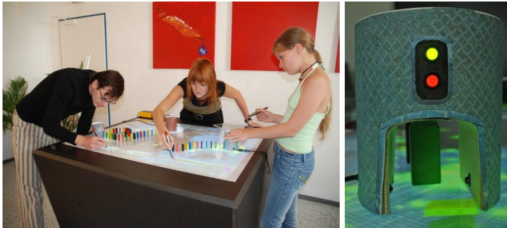
Figure 13: (left) Players have to draw a path on the surface for placing digital domino tiles. (right) Different physical objects have to be used for pushing the real/digital domino pieces. The photo sensor of a tower, for instance, can track the falling physical piece and push the digital ones.
