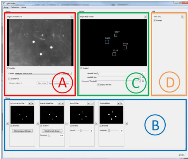
Figure 2: The four plugin sections of the LightTracker: The image created by the source (A) is processed by the filter chain (B), analyzed by the tracker (C), and the resulting blobs, after conversion by the calibration, are forwarded to the application by the sink (D).
