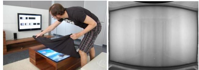
Figure 9: The calibration process for the intensity map filter (left) and the resulting reference image illustrating the uneven lighting situation (right).
