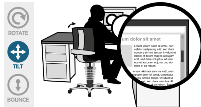
Figure 3. Example for a manipulating (tilting) gesture to control scrolling of web content in a browser.
