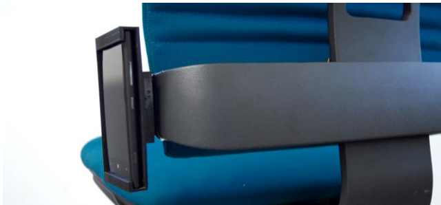
Figure 3. Smartphone sensor attached to the backrest of the 3DDee™ flexible chair.
