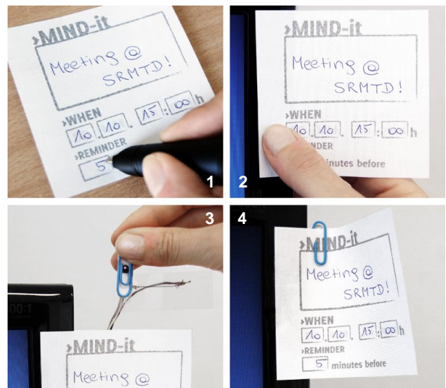
Figure 2: Handwritten notes are captured on paper (1), stuck to a prominent location (2), and combined with a technologically enhanced paperclip (3) that triggers motion feedback (4).
