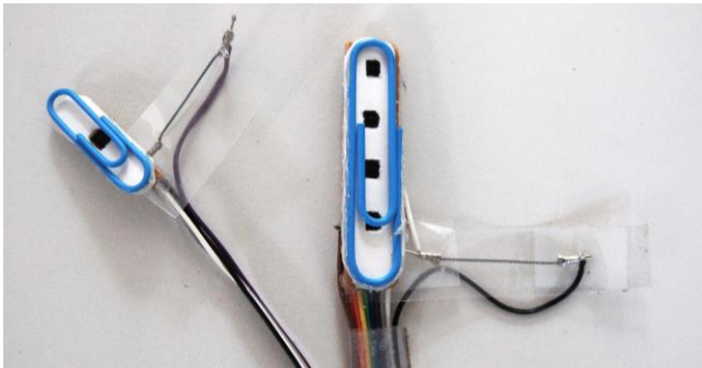
Figure 3: A Move-it mono-sensor (left) and multi-sensor (right) ioClip with reflective sensors for sticky note identification and SMA for actuation.
