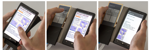
Figure 11. Clipboard. Left: A recommender app is temporarily opened. Middle: Content in the recommender app is copied onto the secondary screen by simultaneously tapping the content and the secondary screen. Right: Text and image are pasted into an e-mail app.
