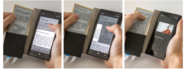
Figure 10. Document Reader. Left: The user can flip through the pages of a document on the LCD by bending the flexible display. Middle: A page gets selected by touch on the LCD and gets pushed over to the secondary e-paper display. Right: The fidelity of the LCD screen can be utilized to show rich media linked in text pages on the e-paper display.
