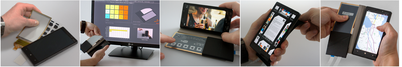
Figure 1. FlexCase is a novel flip cover for smartphones, which combines a flexible sensor and e-paper display to enhance interaction with existing mobile phones. The cover can be used in a variety of configurations and it augments phone's existing input and output capabilities with a variety of new interaction techniques, such as bimanual and back-of-device interaction or the incorporation of different grips for mode-switching.
