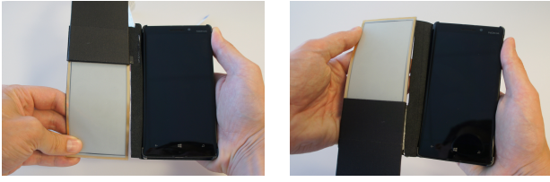
Figure 3. The final layout was evaluated with early mockups. For ergonomic reasons, given the hand position and hand mobility, we decided for arranging the display at the top left side of the flip cover (Right).
