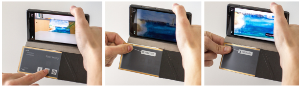
Figure 13. Camera. Capture settings are visualized on the secondary screen, leaving the primary display free of clutter. Functions, such as flash settings (Left), can be activated via touch or linear parameters, such as aperture (Middle) or exposure (Right), can be selected and controlled with different grips.
