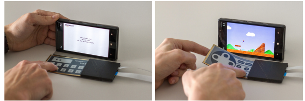
Figure 14. Left: Input of a combination of digits and pressure information for increasing security in public areas. Right: Showing a flexible gamepad layout with touch-enabled buttons and bend sensing.
