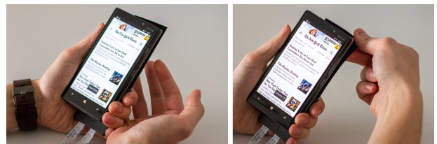
Figure 15. Left: A swipe gesture on the back of the device plays the next song in a music player running in the background. Right: The volume is adjusted with a corner Grip & Bend gesture.
