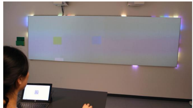
Figure 9: Setup in experiment two: On the tablet the target note is shown. Glowworm refers to the chains of colored lights.
