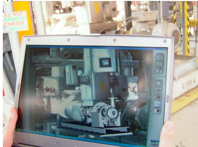
Figure 5: The OMV demonstrator application shows the inner parts of a pump.
