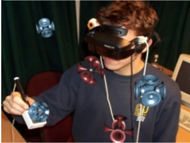
Figure 2: A user can place with ASR different sound sources in the real world and he can play them in 3D.
