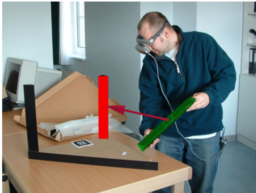
Figure 7: The user can use an HMD to get the necessary information where to place the next wooden feet of the table.
