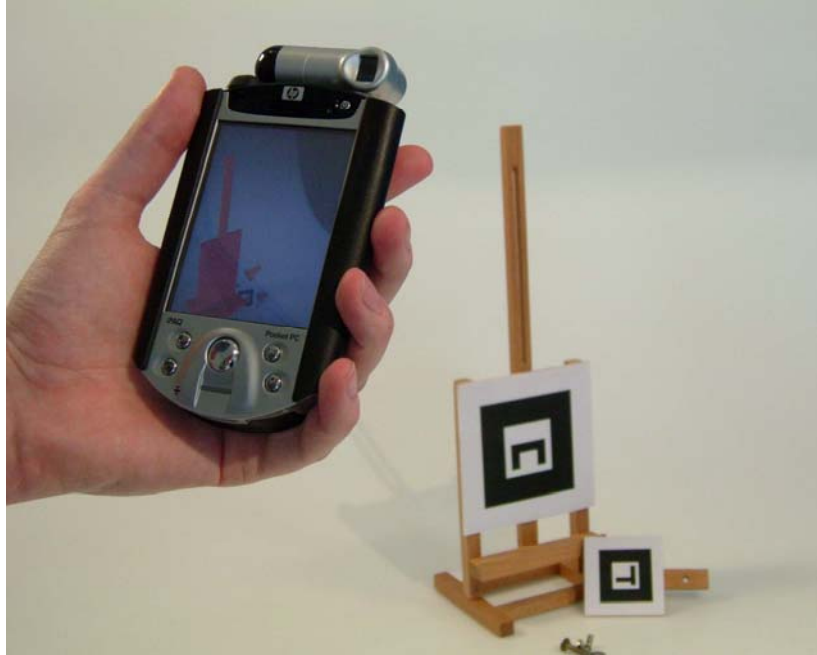
Figure 6: The PDA version of FaiMR shows a simplified step-by-step assembly instruction example.
