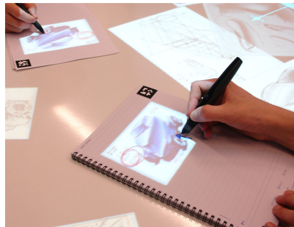
Figure 1: Videos, images, and 3d objects can be projected on the paper and be combined with annotations made with the digital pen.
