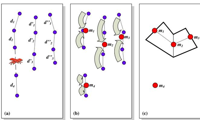
**Figure 13: The pipeline of the specular highlight: after merging the particles ( $p_i$ ), we achieve potential points  $m_i$  (b) which are representing potential points for creating the triangle mesh (c).**
