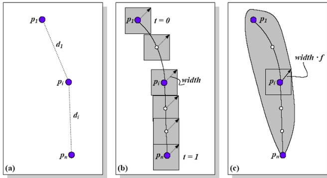
**Figure 3: Creation of a hair strand: With user-defined particles (a), we define a Catmull-Rom spline on which the billboards are generated (b). Finally, the width of the billboard is re-sized to guarantee a better shape for the strand (c).**
