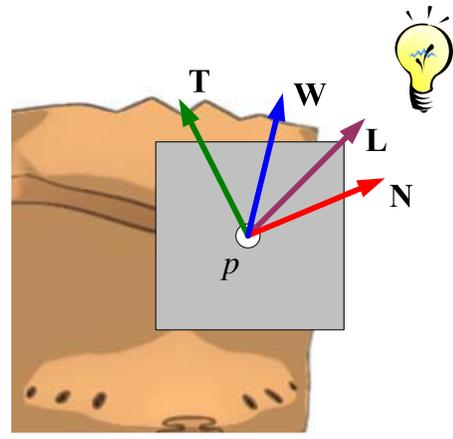
Figure 11: Calculating the specular term.
