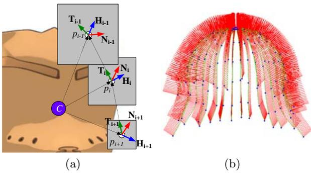
**Figure 6: Calculating the normal vector:** (a) The tangent vector and the vector with its origin in the head’s center are used to calculate the right vector. (b) The cross product of the right vector and the vector  $T_i$  are then used to calculate the normal vector.
