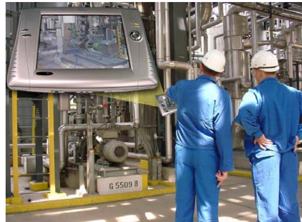
Figure 2: In AMIRE a refinery employee can explore the environment with a Tablet PC and mixed reality technology.
