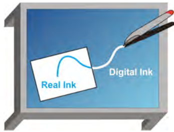
Figure 2. A hybrid pen writes with real ink on the palette surface and acts as digital input on the augmented tabletop (which is covered with an ink-repellent layer)
