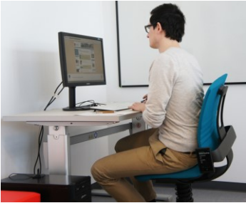
Figure 5. A user controlling a PC through the movements of his body while sitting on a flexible office chair, e.g., tilting, rotating, bouncing.
