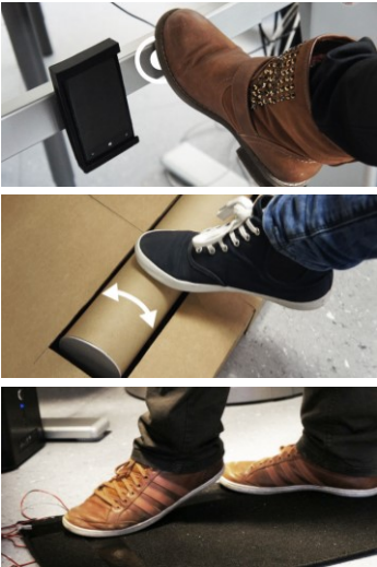
Figure 6. A user controlling a PC through foot gestures, e.g., kicking, rolling, tapping, swiping.
