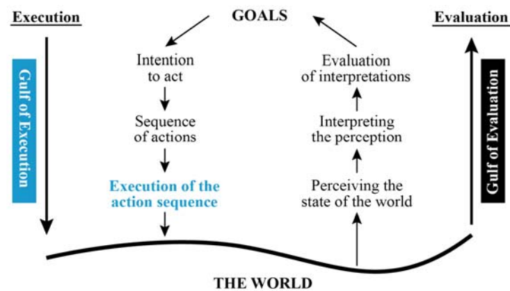
Fig. 9.4 Seven Stages of Action: The Stages of Execution start at the top with the goal, the state that is to be achieved. The goal is translated into an intention to do some action. The intention must be translated into a set of internal commands, an action sequence that can be performed to satisfy the intention. The action sequence is still a mental event: nothing happens until it is executed, performed upon the world. The Stages of Evaluation start with our perception of the world. This perception must be interpreted according to our expectations and then evaluated with respect to both our intentions and our goals (reproduced from (Norman 2002))
