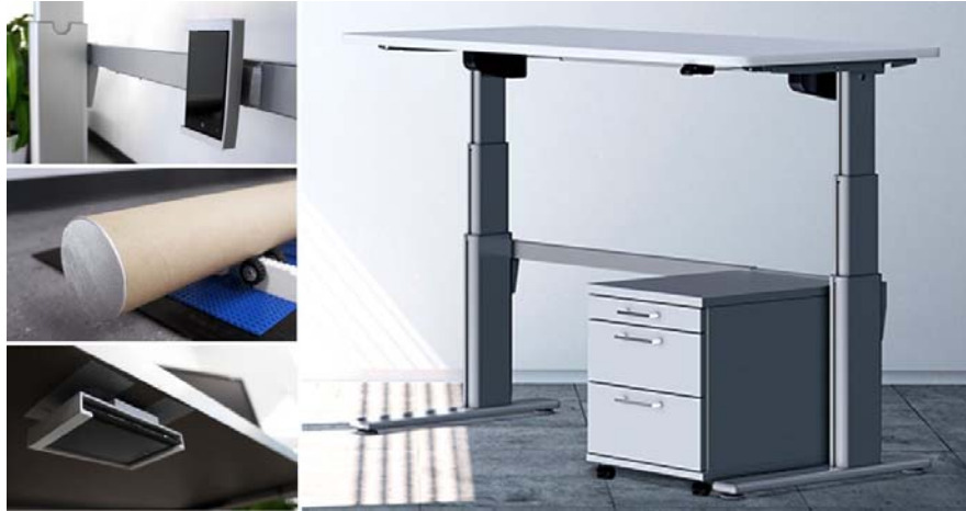
Fig. 9.8 Prototypes for peripheral interaction through smart furniture: smart furniture modules for under-the-desk kicking, rolling, touching.
