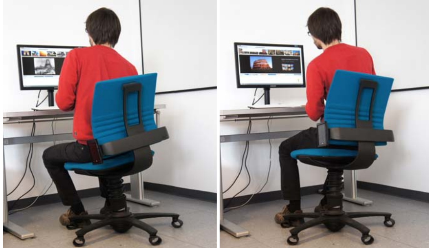
Fig. 9.10 Peripheral interaction through smart furniture: rotating, tilting, and bouncing gestures on an interactive flexible office chair.
