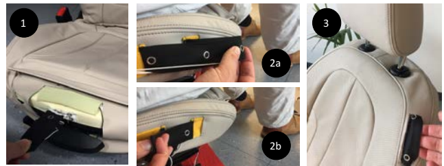
Figure 16: Adjusting the car seat position by stretching the StretchEBand sensor.
