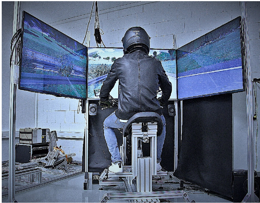
Fig. 3. Electric scooter riding simulator at WIVW.
