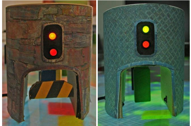
Figure 3: Different physical objects have to be used for pushing the real/digital domino pieces. The actuator of the first tower can push real domino tiles. The photo sensor of the second tower can track the falling physical piece and push the digital ones.
