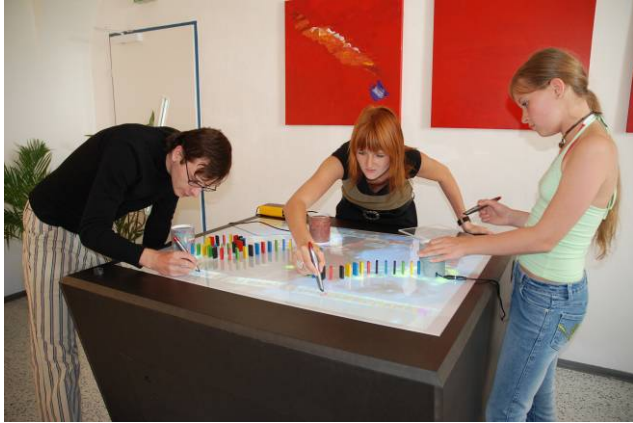
Figure 5: Comino in action. Up to four people can interact simultaneously with the system and place both real and digital domino tiles.
