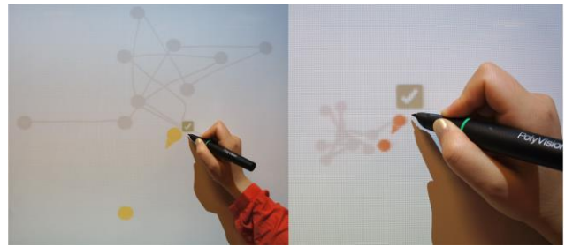
Figure 5: Experiment tasks in Large (left) and Small (right) scales. The check icon on each condition is the feedback provided when a designated color switch is successfully performed
