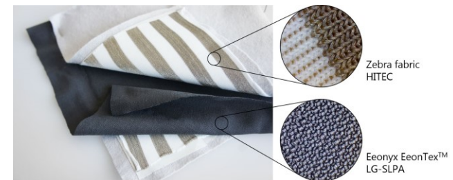
Figure 2. FlexTiles consists of a sandwich design of two electrode layers and a force sensitive layer in between.
