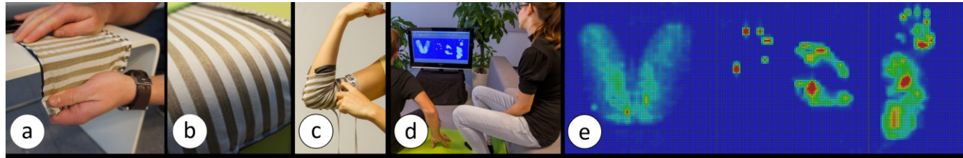
Figure 1: FlexTiles is a thin, flexible, stretchable and form-fitting pressure-sensitive tactile input sensor for sensing complex 3D shapes (a-c). It also enables the measurement of large areas like a couch in real-time (d-e).
